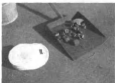
图9 “设计 A”型避雷器未通过短路电流试验 Fig.9 Design “A” surge arrester did not pass the short-circuit test
